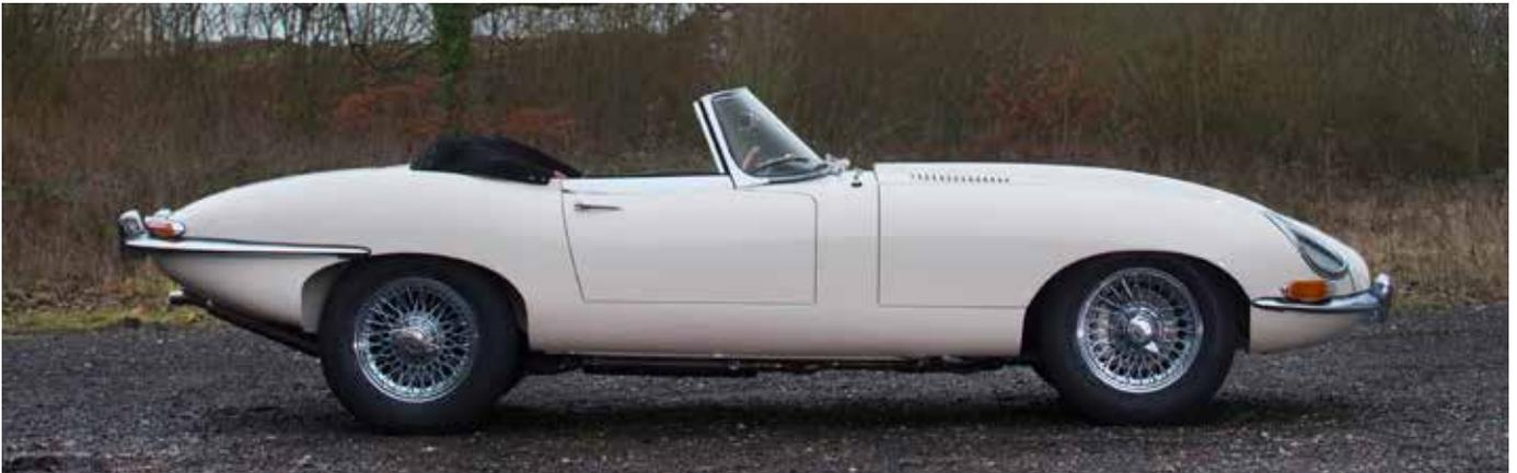
Introduced in 3.8-litre form in 1961, the E-Type caused a sensation when it appeared, with instantly classic lines and 150mph top speed. The newcomer's design owed much to that of the racing D-Type: a monocoque tub forming the main structure, while a tubular spaceframe extended forwards to support the engine. The latter was the same 3.8-litre, triple-carburettor 'S' unit first offered as an option on the preceding XK150.
